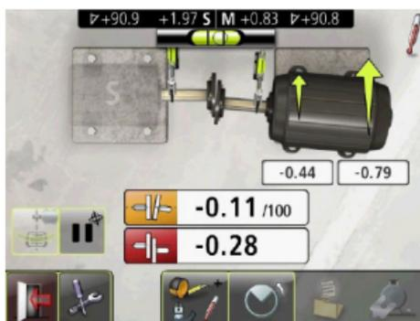
**5.** Continue to adjust the movable machine, watching the live readings, until both the angle and offset are within tolerance.
