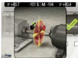
**4.** Make the largest adjustment first. The arrows indicate the direction of adjustment.
