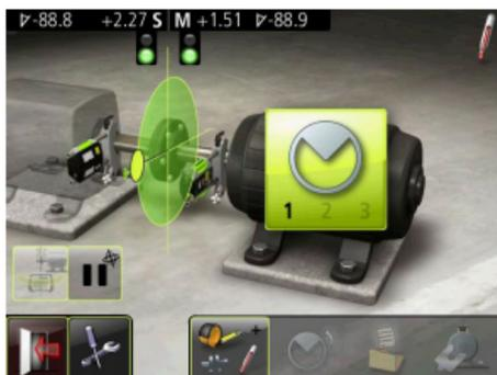
**5.** Rotate the sensors to the 12:00 position, being sure they move outside the red portion of the circle on the screen. Press the measurement button again to take the second measurement.
