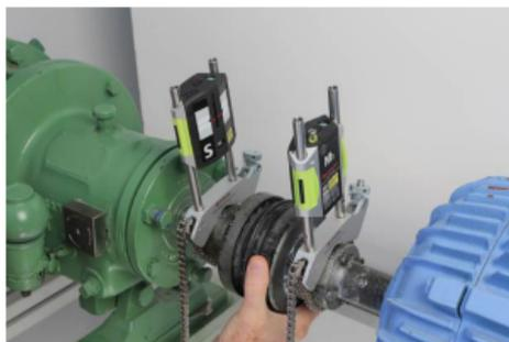
**6.** Rotate the sensors out of the red portion of the circle towards 3:00.
